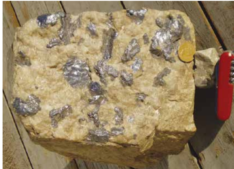
Molybdenum rosettes on vein surface. Sample was taken from underground workings excavated for metallurgical bulk sample extractions by past operator.
